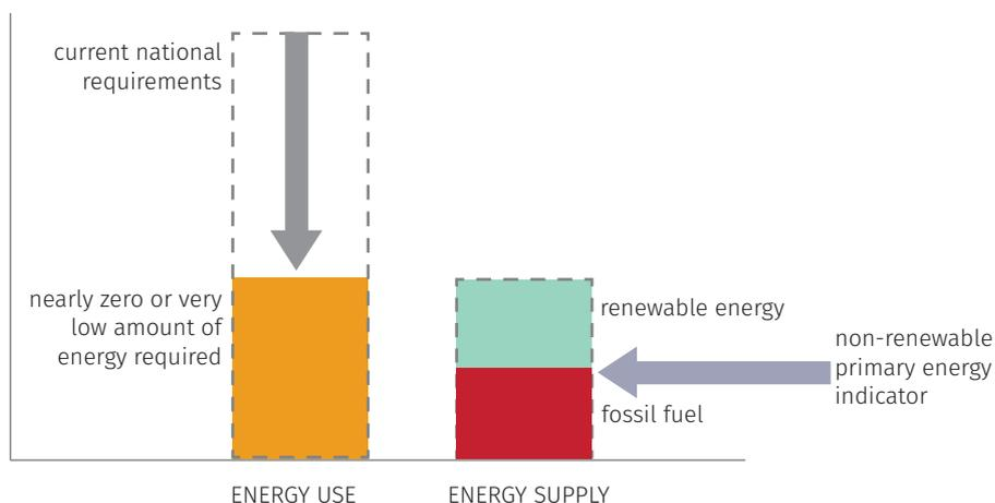
Figure 1: Graphical interpretation of the NZEB definition according to Articles 2 and 9 of the EPBD [4]
